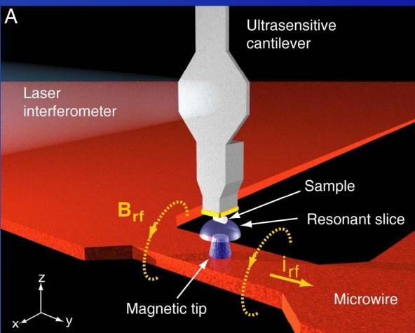
Sensing the force between a magnetic tip and nuclear-spins on the cantilever
