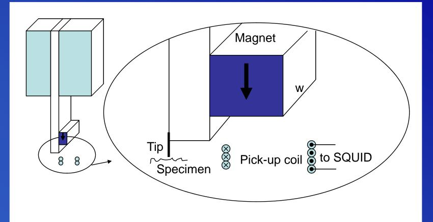
Superconducting Quantum Interference Device: Most sensitive magnetic detector
