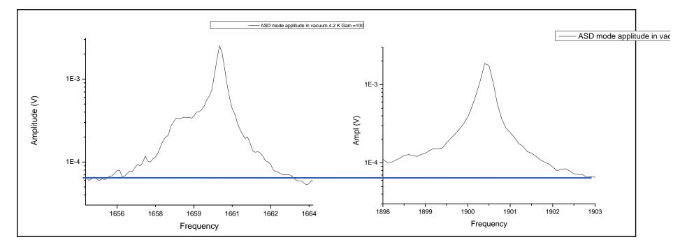
Without driving resonances are measured around 1660 Hz and 1900 Hz. detection noise floor 40 pm/sqrt(Hz)
