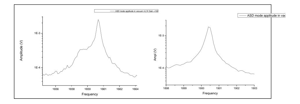
Without driving resonances are measured around 1660 Hz and 1900 Hz. detection noise floor 40 pm/sqrt(Hz)
