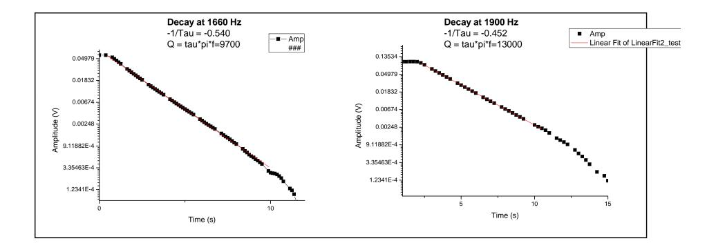
Without driving resonances are measured around 1660 Hz and 1900 Hz.
